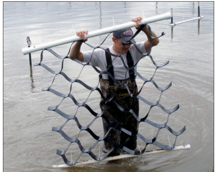
Figure 3. Sections of plastic geoweb used as spawning substrate. Plastic pipe was used as a float, and a small diameter pipe filled with sand served as a weight.
